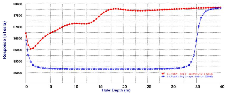
*The plots show the variation in the 3 orthogonal responses along the borehole between the vertical and dipping hollow casing.*
