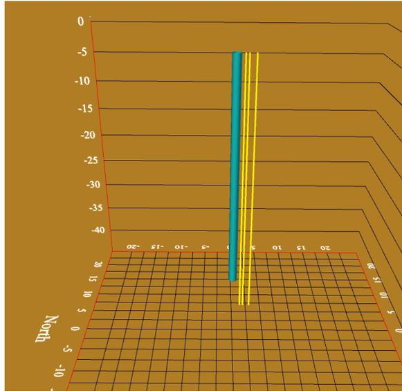
The model of the casing, shown to the left, has a susceptibility of 50 (SI units), and is 1.32 m in diameter and 35 m long. The top is located just below the surface (0.01m).
