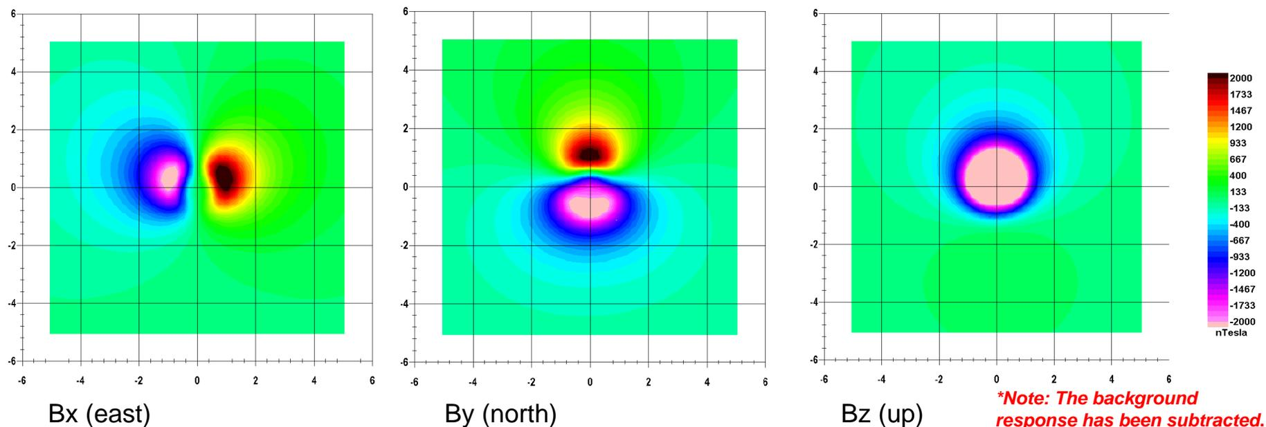
**5 m x 5 m plan view:** Response on a plane 0.5 m below the object. Same scale for all components for a casing with high susceptibility. These figures show clearly the nature of the near-field, strong scattering effects of the casing. Bz is essentially a monopole rather than a dipolar response while Bx,By are distorted dipoles rather than quadrupoles as they would be in the weak scattering case.
