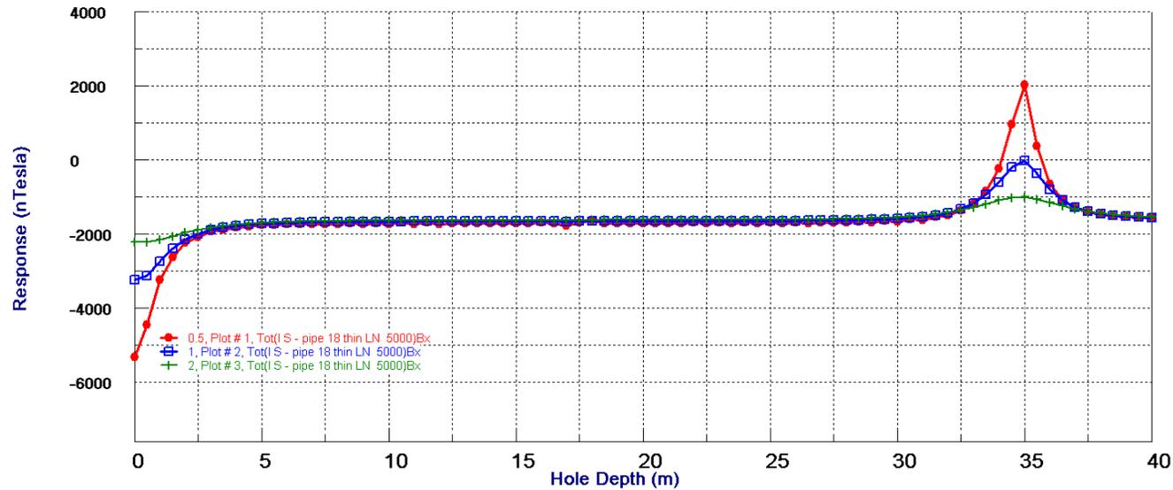
**Response of hollow target in the borehole.** Comparison of responses in boreholes at different distances from the target. There is very little difference in the responses except at the top and bottom of the boreholes.
