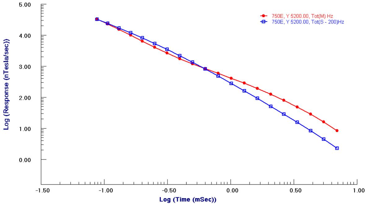
Plot measured data against model as a quick check. This simple half-space model does not fit the details of the decay but the amplitude is as expected. Proceed with further modeling, or inversion, as desired.
