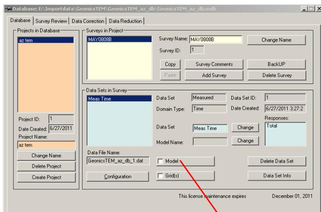
It is recommended that you build a simple layered earth model with a reasonable resistivity for the site to check the data. i.e., verify that the data was imported properly (correct units, etc) and the system was set up properly. Also check that the sign of the data matches that of the simulation.
