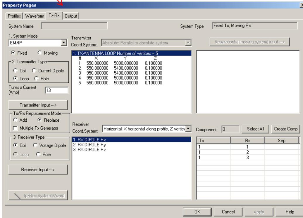
On the Tx-Rx page, the details of the transmitter and receiver are specified, as well as the separation (for a moving system).
