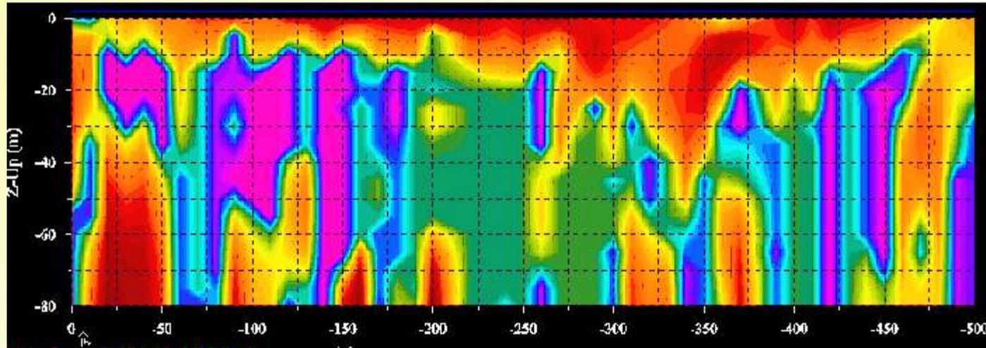
Depth of Investigation Set to 60m. Log Apparent Resistivity vs Depth
