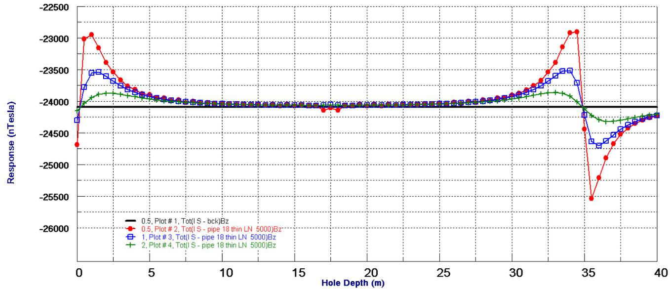
Comparison of the response of the hollow cylinder in three boreholes at different distances from the target.
