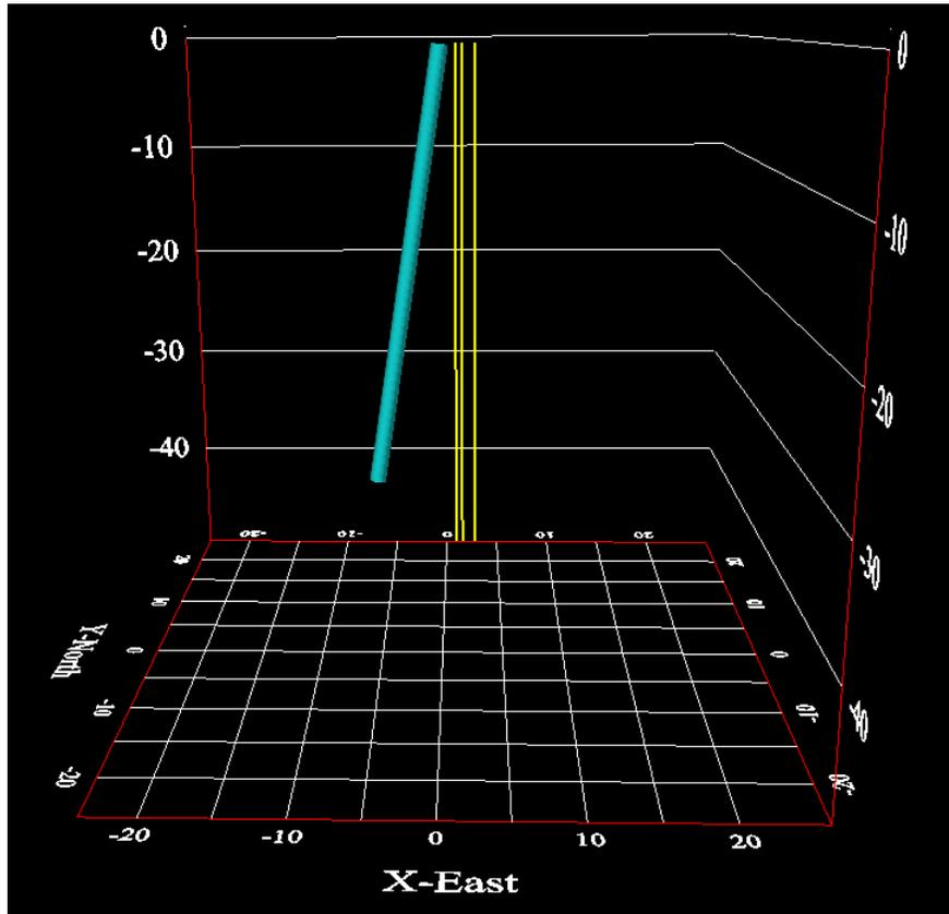
The dipping casing has the same dimensions, but is now dipping at 81.5 degrees to the west.
