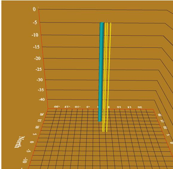
The model of the casing, shown to the left, has a susceptibility of 50 (SI units), and is 1.32 m in diameter and 35 m long. The top is located just below the surface (0.01m).
