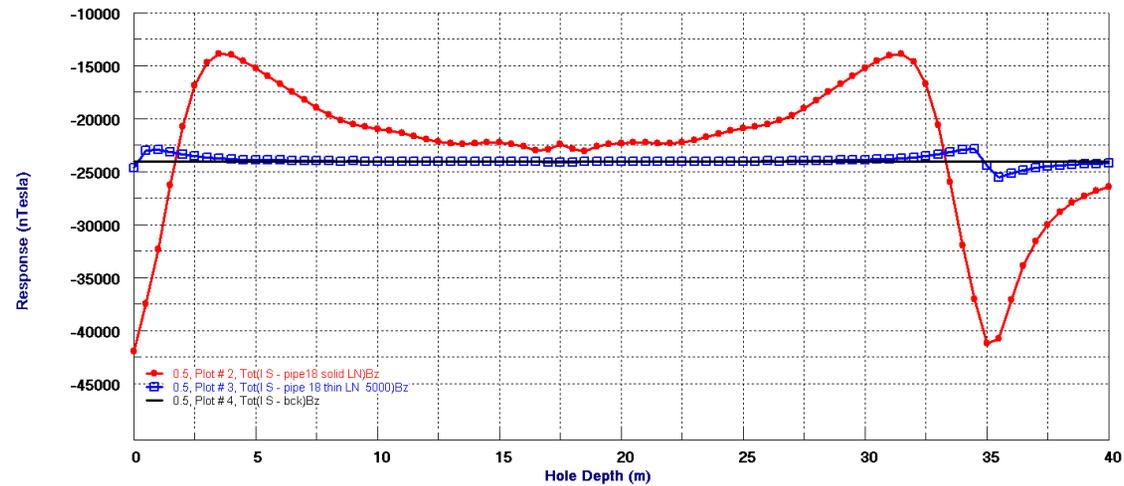
Solid cylinder (**red**) vs hollow cylinder (**blue**) along a borehole 0.5 m away from the edge of the casing.
