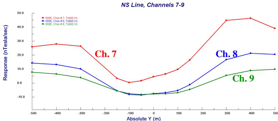
The ground TEM data used a fixed loop of about 400 m by 400 m. Measurements were taken along a north-south and an east-west line running through the center of the loop. There were 7 stations inside the loop and 6 stations outside the loop along each line. Asymmetry inside the loop can be observed along both lines at early times, suggesting 3-D structure. The response inside the loop was smaller than the response outside the loop beginning at mid-times. This may be due to a system response.
