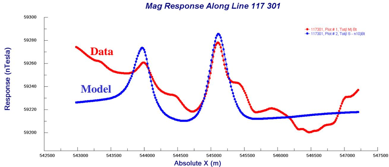
A rough model for the aeromagnetic data over Wolf Creek was developed to determine the location and approximate properties of the structures causing the two main anomalies in the magnetic response. These features are long, narrow, fairly shallow, and have susceptibilities from 0.035 to 0.06. The magnetic model was used to assist with the modeling of the TEM data.
