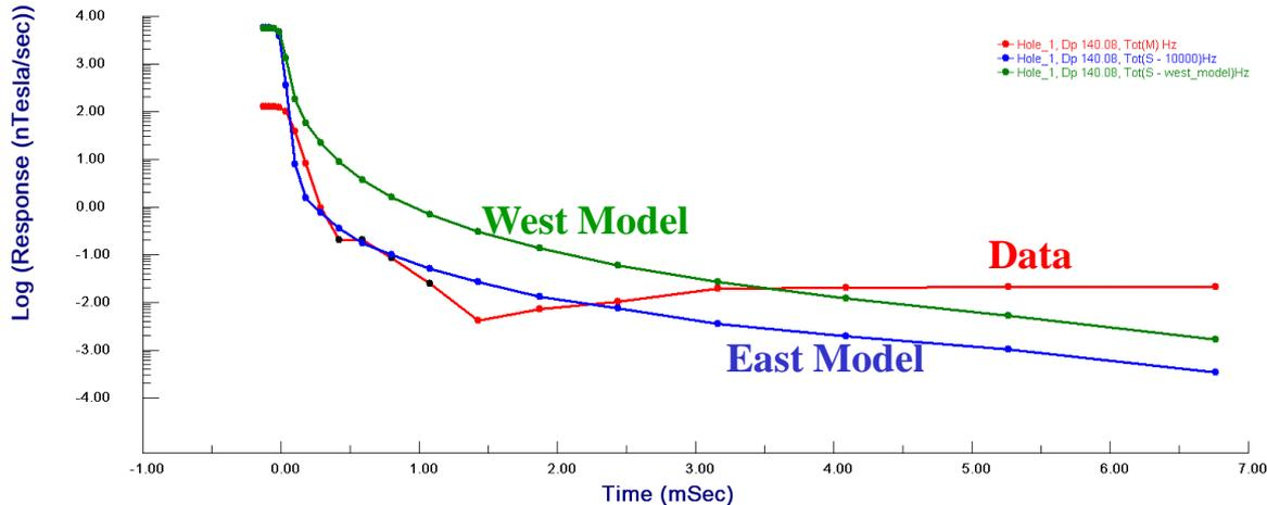
The borehole TEM data fo HB-05-19 is modeled fairly well by the east model throughout the borehole. However, the amplitude of the east model is too low for the ground data, which is better modeled by the west model.
