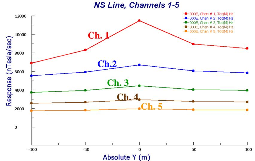
The ground TEM data used a fixed loop of about 400 m by 400 m, centered on the borehole. Measurements were taken along a north-south and an east-west line running through the center of the loop. The stations were symmetric about the center. There were 5 stations inside the loop along each line, and 6 stations outside the loop along the EW line. Along the EW line, the response inside the loop was smaller than the response outside the loop at late times, possibly due to a system response.
