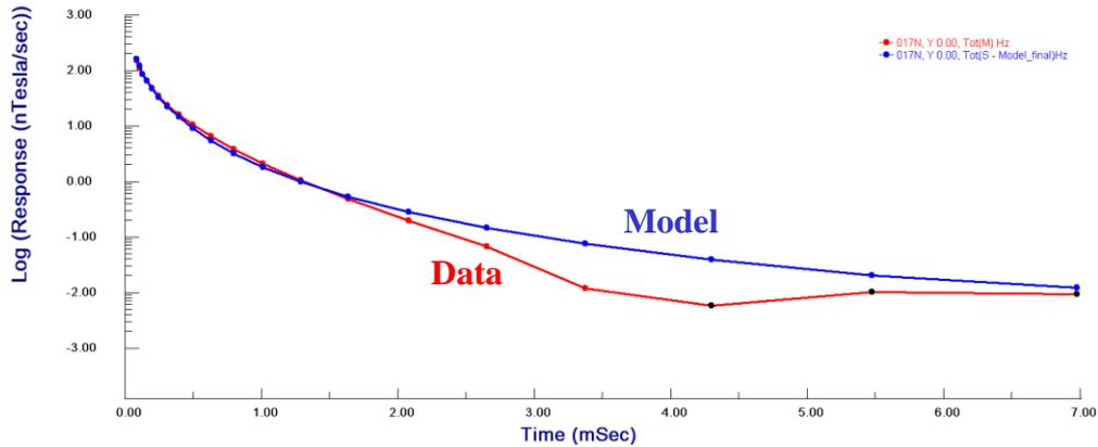
The ground model for S-17 contains sandstone and less resistive sandstone with mudstone interlayers above the basement. The amplitude of the ground model is too large for the MegaTEM data, but the discrepancy is not as large as it is for HB-05-12 and HB-05-13.
