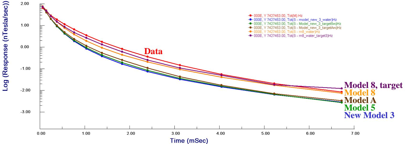
The amplitudes of the responses for Model A and Model 5 are too small for the ground data. The previous layered earth model, Model 8, fits the data much better. When a long, horizontal target was added at -440 m to Model 8, the response fit the data slightly better than Model 8; however the amplitude of the curve was too large for the airborne data
