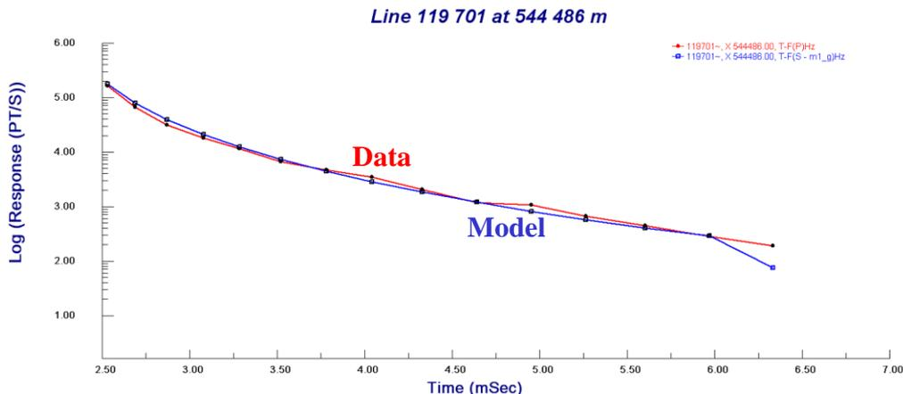
A model was developed to fit the airborne data. Some of the resistivities at depth in the ground model were increased, and a good model was obtained. However, the amplitude of the response for the model is too low for the ground data, even with a conductive layer overtop to account for possible water at surface when the ground data was collected.
