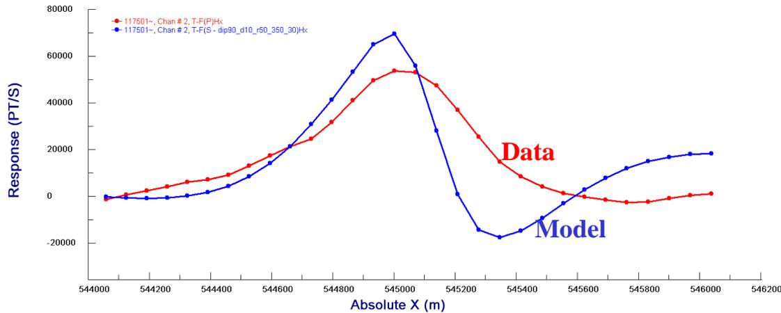
The prism in the magnetic model that causes the eastern anomaly was used to model the TEM data. The prism was inserted into a simple layered earth model with a 500 m thick, 1000 Ohm m layer over a resistive basement. Its properties were adjusted so that it matched the TEM data more closely. It was found that a model containing a narrow prism with a resistivity of 50 Ohm m, a dip of  $90^{\circ}$ , and a dip extent of 350 m fit the response near the contact fairly well.
