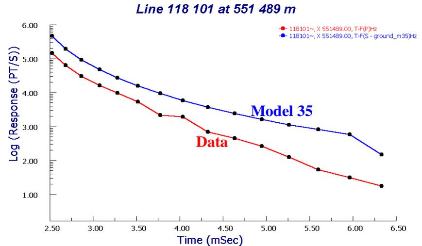
The first five measurements were taken in the on-time, and were not used for modeling. The sign of the airborne data was flipped to match the current direction of the model.
