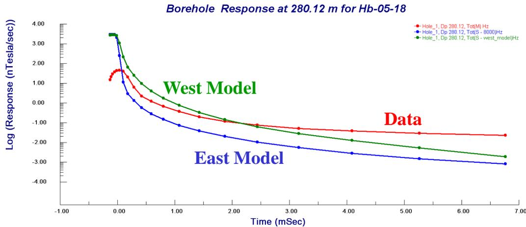
The west model developed for the MegaTEM data fits the borehole data for HB-05-18 fairly well near the bottom of the borehole. The east model (resistive half-space) fits the borehole data better at shallower depths.
