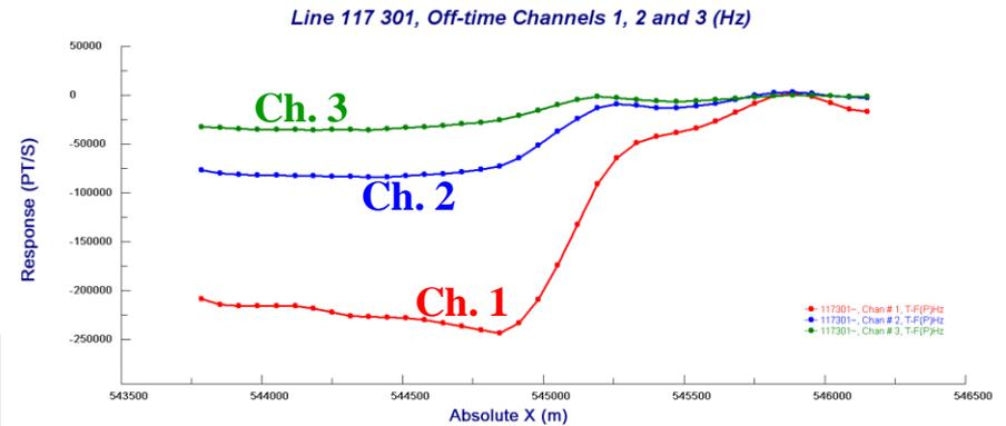
The MegaTEM data also suggests structure in the Wolf Creek area. As observed in a contour plot for off-time channel 3 (time channel 8), there appears to be a contact or fault around 545 000 m. The plots show a change in the amplitude of the response around this point.
