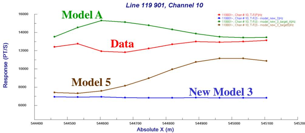
Based on the Marquardt inversion, a target was added to the new layered earth model, which increased the response of the model. Model A contains two flat plates at 600 m depth. Model 5 contains a dipping plate.
