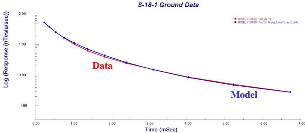
The ground model for S-18-1, developed using a Marquardt inversion, contains a resistive sandstone layer and a conductor underlying the basement. The amplitude of the ground model approximately the correct amplitude for the MegaTEM data.
