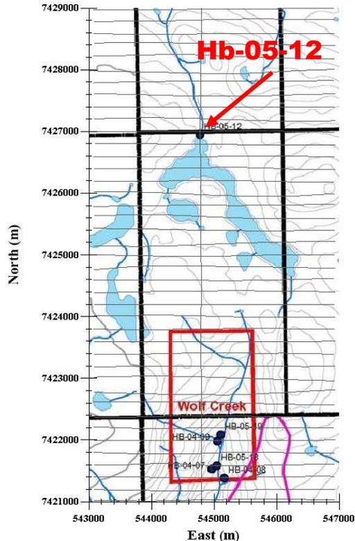
Ground TEM , borehole TEM, and airborne TEM (MegaTEM) data collected near HB-05-12 were studied. The data were used to investigate the variation in resistivity with depth. To develop a layered earth model, forward modeling was performed, with the user creating a model, comparing the synthetic data to the TEM data, and modifying the model as needed. Good models were compared with all sets of data, as an appropriate model should fit the ground, borehole and airborne TEM data.
