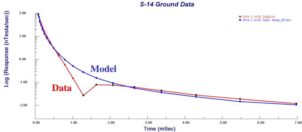
The ground model for S-14, developed with the assistance of a Marquardt inversion, contains a resistive sandstone layer above the basement and a conductor underlying the basement. The amplitude of the ground model is slightly too large for the MegaTEM data.
