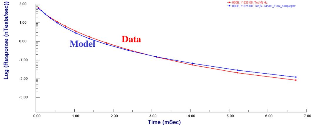
The previous model was simplified to develop a new model with a very similar response. However, the amplitude of the model is too large for the airborne data, although the shape is similar. Profile plots of the data, which are fairly symmetrical, do not suggest the presence of a significant target, and adding a small target makes the response much too large at early-mid times.
