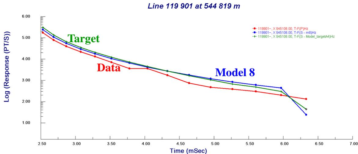
The new layered earth model was modified so that it would fit the ground data better. A target, like the one that was added to Model 8, was put into the new layered earth model. This new model not fit the data better than Model 8. Additional modeling may assist in developing a slightly better layered earth model and target to fit the different types of data; however, it has been very difficult to find a model that matches both the airborne and ground data in current modeling.
