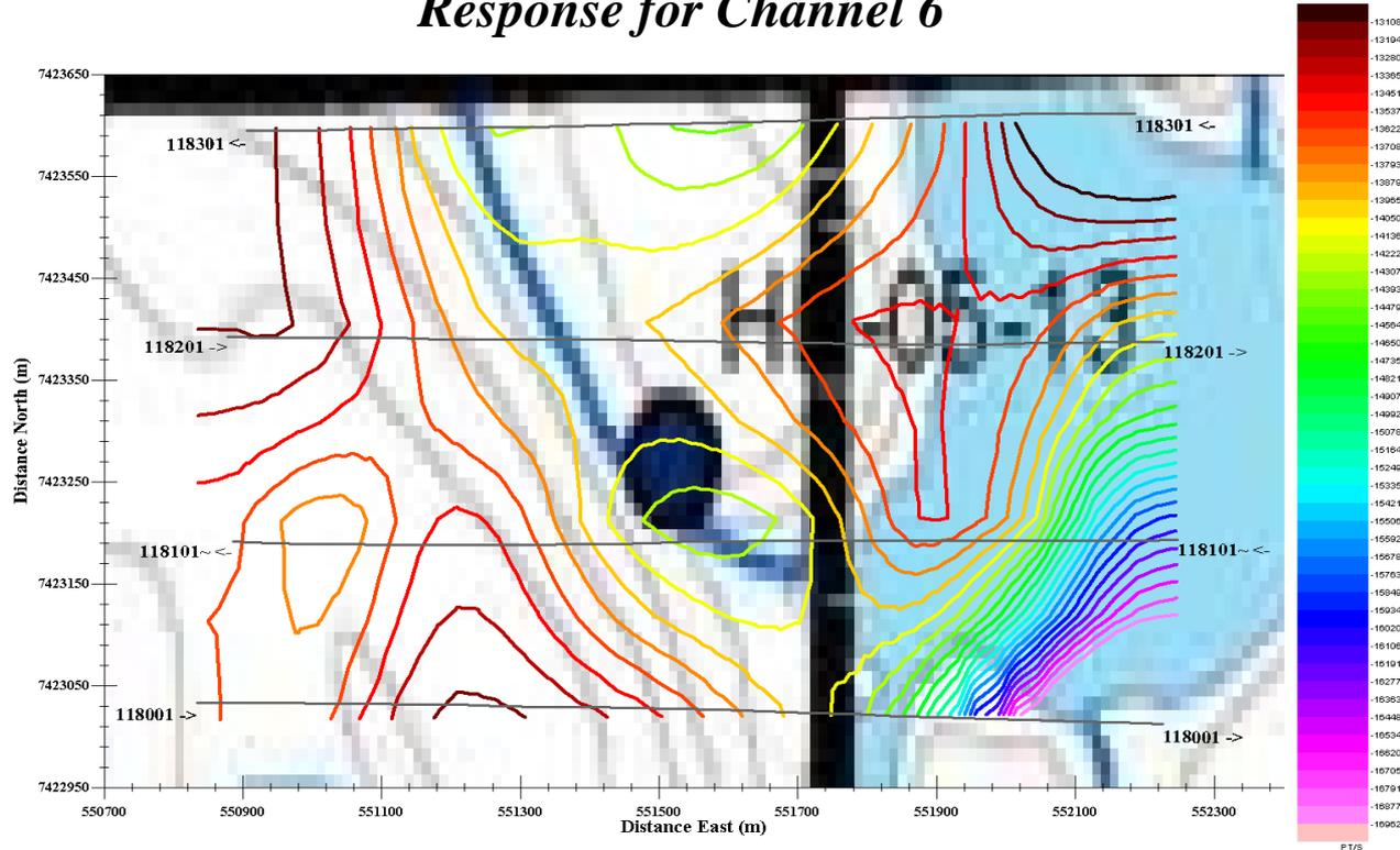
A MegaTEM survey was flown over the Coppermine River Region, and a focus area comprising part of the 4 lines around HB-05-13 was cut out for the purpose of comparing it with the ground data.
