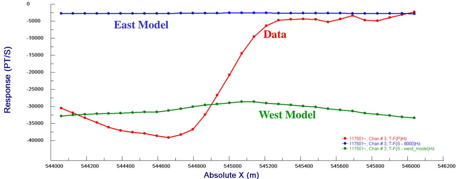
Initial modeling focused on developing separate layered earth models for the east and west sides of the region. The response on the east, which has a lower amplitude, was modeled by a half-space with a resistivity of 8000 Ohm m. To the west, the response was modeled by a 500 m layer with a resistivity of 1080 Ohm m above the basement, which has a resistivity of 8000 Ohm m.
