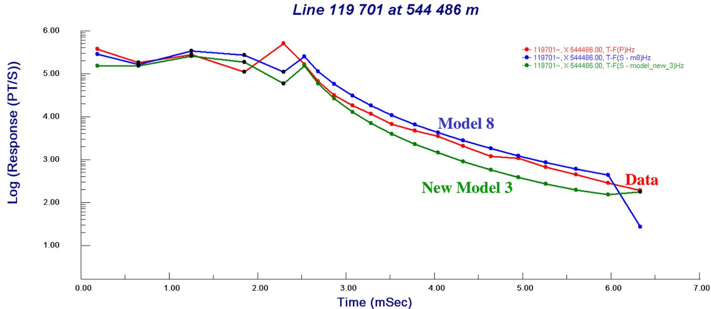
Based on the results of the inversion, a new layered earth model was developed, containing a less resistive overburden and higher resistivities at depth. As shown in the decay curves, this results in a lower response than Model 8.
