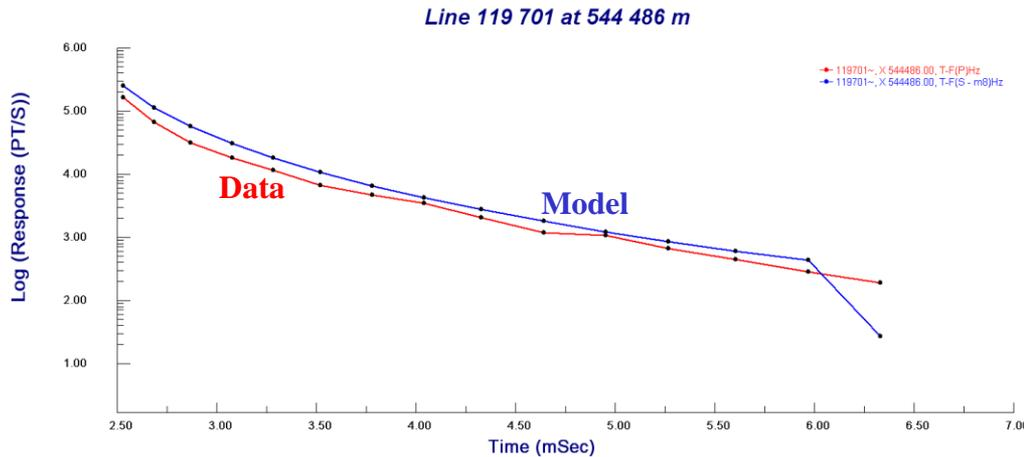
Further modeling focused on finding a model to fit both data sets. A thin conductive layer was added to the model for the ground data to raise the amplitude of the response. An overall better model (Model 8) was found; however, the amplitude of the response from the model is too large for the airborne data, and still too small for the ground data.
