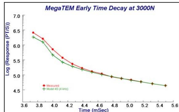
Figure 4: Early-mid time Hz decay on Line 10090 at (700E, 3003N) in the MegaTEM. Red is the measured data. Green is the response of Model 4S for a receiver bandwidth of 4 kHz.
