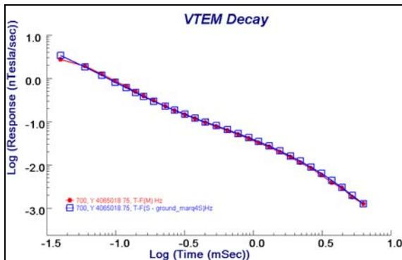
Figure 5: Decay on Line 700 at (690E, 5018N) in the VTEM, after waveform adjustments. Red is the measured data. Blue is the response of Model 4S for the initial simulation settings.
