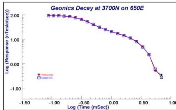
Figure 1: Hz decay at 3700N on Line 650E in the Protem ground data. Red is the measured data. Blue is the response of Model 4S.
