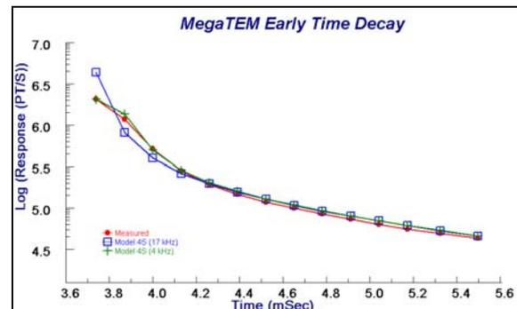
Figure 3: Early-mid time Hz decay on Line 10090 at (700E, 4812N) in the MegaTEM. Red is the measured data. Blue is the response of Model 4S for a receiver bandwidth of 17 kHz. Green is the response of Model 4S for a receiver bandwidth of 4 kHz.
