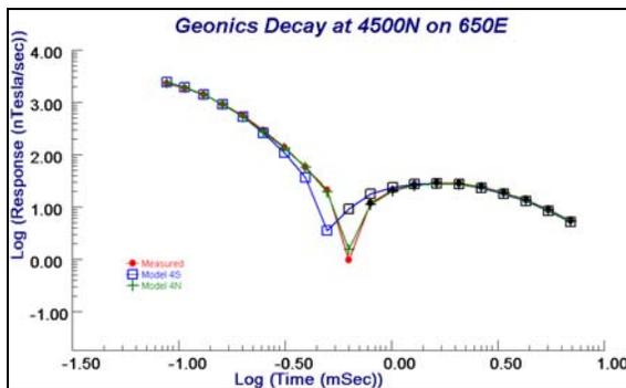
Figure 2: Hz decay at 4500N on Line 650E in the Protem ground data. Red is the measured data. Blue is the response of Model 4S, and green is the response of Model 4N.
