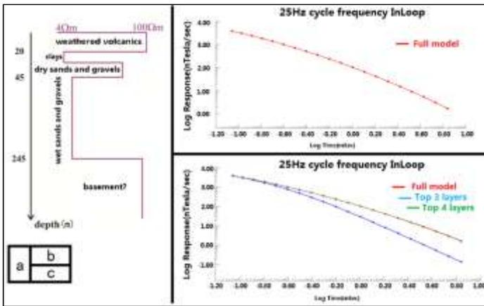
Fig. 3. Comparison of in-loop data from standard model vs similar models
