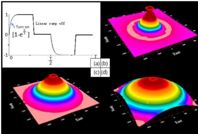
Fig. 1. Current migration underground reflected in a surface of Hz
