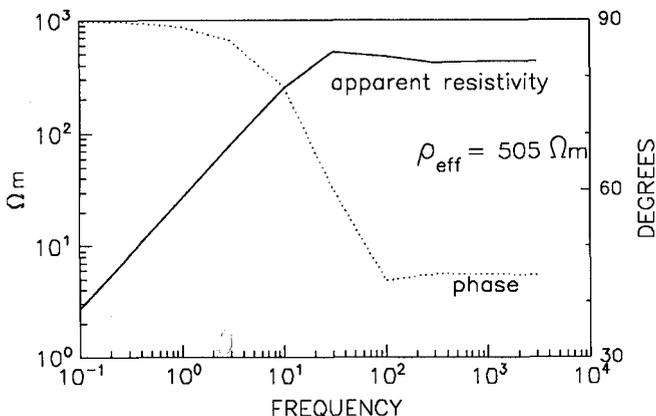
FIG. 7. Fine structure impedance with 110 m electrode. In this model  $d = h = 10$  m while again  $\rho_h = 1000 \Omega\text{m}$  and  $\rho_a = 10 \Omega\text{m}$ . The electrode covers five doublet pairs and one more conducting structure.
