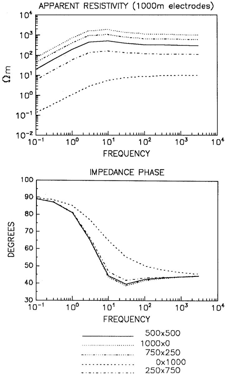
FIG. 6. A study in the use and abuse of long electrodes to measure the electric field. In this model  $d = h = 1$  km, while  $\rho_h = 1000 \Omega\text{m}$ ,  $\rho_d = 10 \Omega\text{m}$ ,  $D = 5$  km and the effective bulk resistivity ( $\rho_{\text{eff}}$ ) is  $505 \Omega\text{m}$ . The electrode length is 1 km and the surface impedances are shown for five different electrode placements.
